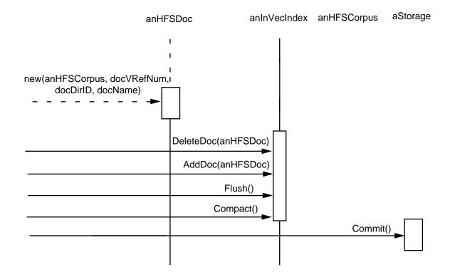
Figure 5-8 Interaction diagram for individual update
